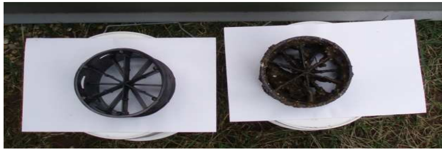
Figure 5: “Coffee can” construction for biofilm growth; the image to the left is prior to microbial growth and the image to the right is after growth.
