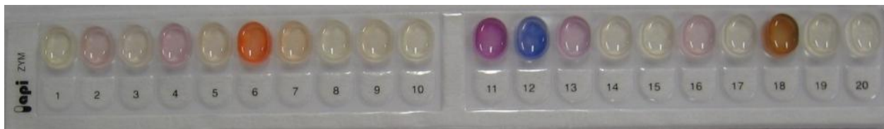
Figure 6: API ZYM – Positive result for enzymatic activity indicated by variable color change.
