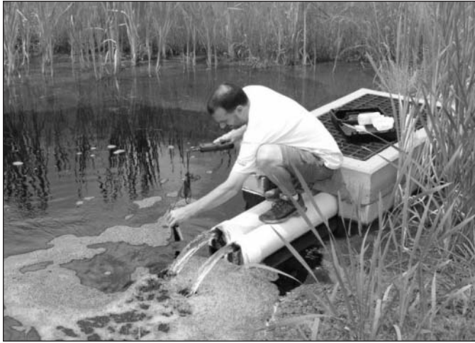
Dr. K's Student Intern John Woodward samples water from a discharge at the BAMR passive treatment facility in the Beech Creek Watershed.
