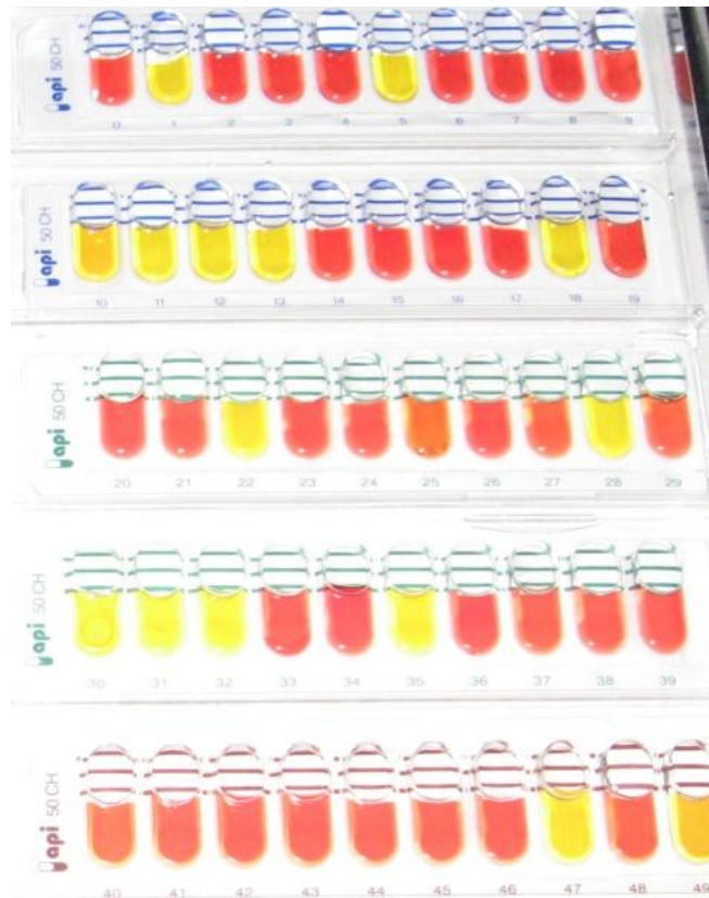
Figure 4: API 50CH – Positive result for carbohydrate utilization indicated by yellow colored cupule. *Results read after 24 hour and 48 hour incubation at 30°C.
