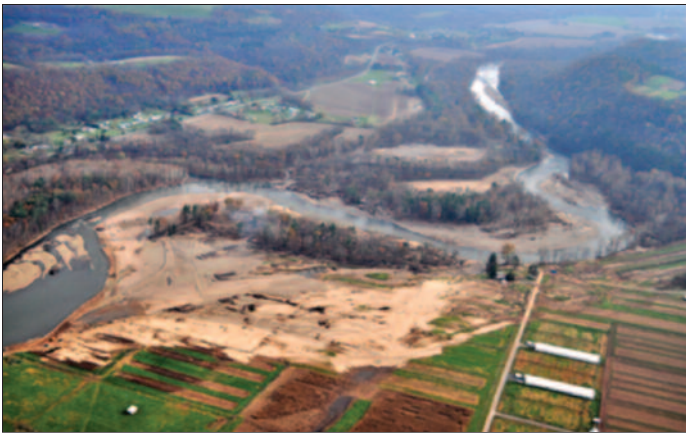
Chute cut through game farm, partly filled with gravel and flanked by 2 m thick sand deposits (Loyalsock Creek).
