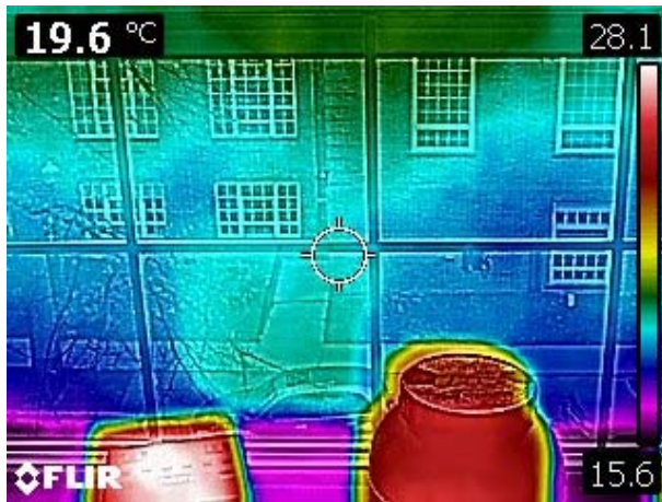
This photo is of room 326: the center of the glass pane is only around 20 degrees C. The cold spot on the bottom is also only 15.6 degrees C
