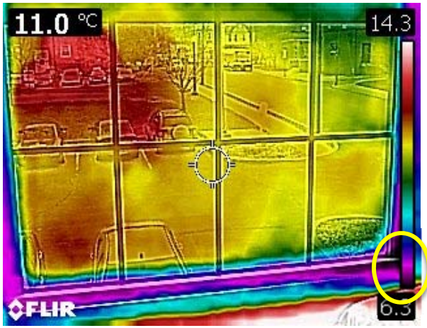
This photo shows room 229: the indicated area of this photo shows an air leak of 6.3 degrees C. as well as the whole base of the window allowing 7 degree C air to infiltrate the room.
