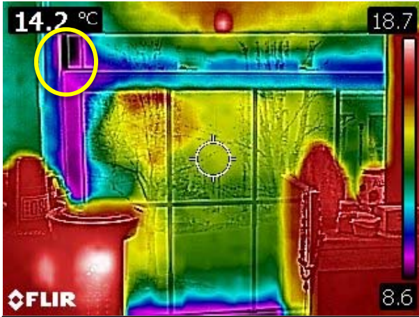
This photo shows room 101: looking at the circled area you can clearly see that there is 8.6 degree C air coming in through the poorly sealed joint in the window. This could be due to a broken or missing gasket
