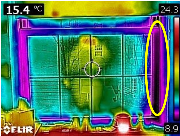
This photo also shows room 101: and in this photo you can see by the indicated area that there is 8.9 degree C air coming in along the right hand side of the window.
