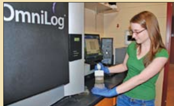
Trisha Duncan '13 is shown pipetting a suspension of bacteria into a 96-well GenIII plate. After incubation in the OmniLog, the results are compared to a database to identify the organism.
